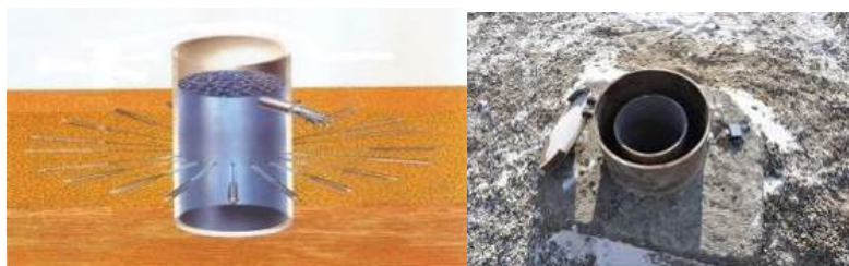
Figure Shallow wells – a water intake option favored by the JETRO Study
