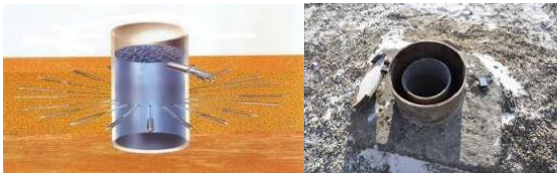
Figure 25. Shallow wells – a water intake option favored by the JETRO Study
